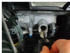
3. Place a container underneath the unit. Place a funnel into the unit and tilt it towards the container to drain the oil.
