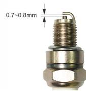
5. Install the spark plugs in reverse order of removal.
