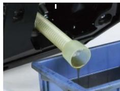
4. Refill oil to the correct level and tighten the dipstick.
