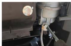
6. Allow the fuel to drain into the container until none remains. Tighten the drain bolt back into place.
