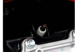
2. Use a ratchet and 5/8 spark plug socket (included with your generator) to unscrew and remove the spark plug.
